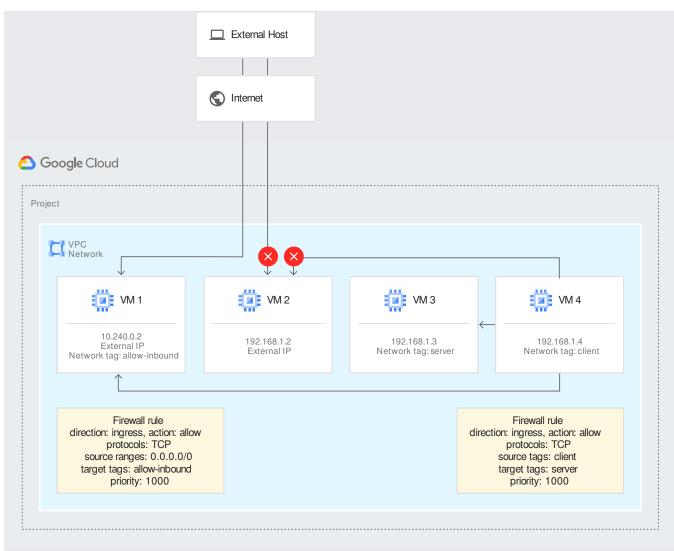
(/vpc/images/firewalls/firewall\_overview\_ingress\_examples.svg) Ingress firewall rules example (click to enlarge)
