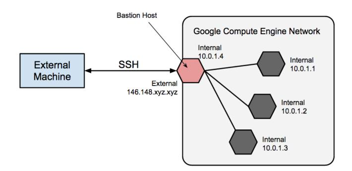
This host can provide a single point of fortification or audit and can be started and stopped to enable or disable inbound SSH. By using a bastion host, you can connect to an instance that does not have an external IP address. This approach allows you to connect to a development environment or manage the database instance for your external application, for example, without configuring additional firewall rules.
