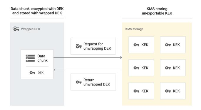
**Note:** Customer-managed encryption keys differs from Customer-Supplied Encryption Keys (CSEK), which let you specify the *contents* of the encryption key. Customer-managed encryption keys let you create and manage a key using KMS, and assign keys to specific resources across Google Cloud. Cloud SQL does not support CSEK.
