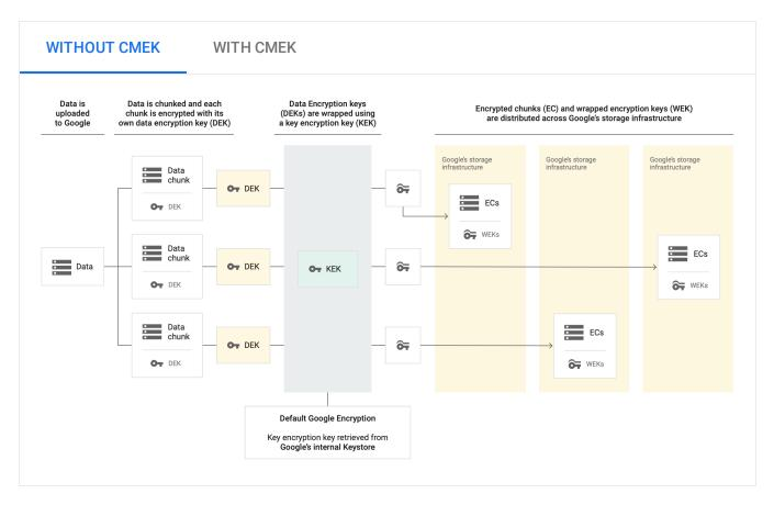
When decrypting data wrapped with customer-managed encryption keys, Cloud SQL uses the KEK to decrypt the DEK and the unencrypted DEK to decrypt data-at-rest.
