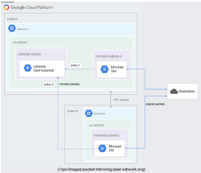
Packet mirroring policies in a central network peered with other networks that have mirrored sources (click to enlarge)
