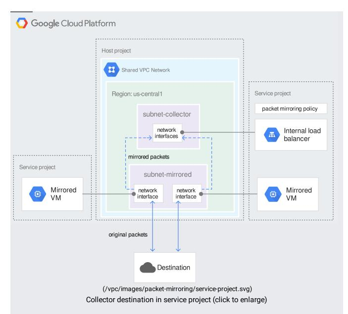
In the preceding diagram, the service project contains the collector instances that use the collector subnet in the Shared VPC network. The packet mirroring policy was created in the service project and is configured to mirror instances that have a network interface in subnet-mirrored.
