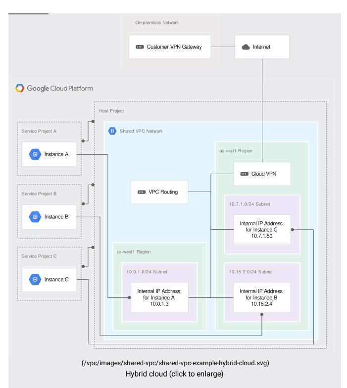
For this example, an organization has a created a single host project with a single Shared VPC network. The Shared VPC network is connected via <u>Cloud VPN</u> (/vpn/docs/concepts/overview) to an onpremises network. Some services and applications are hosted in Google Cloud while others are kept on-premises:
