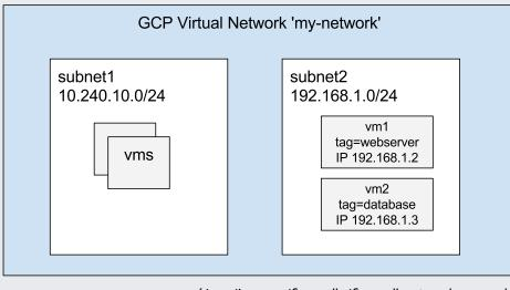
(/vpc/images/firewalls/firewall-network-example.svg) Sample network configuration (click to enlarge)
