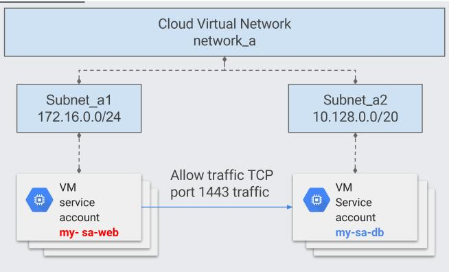
(/vpc/images/firewalls/firewall-service-accounts-example.svg) Using firewall rules with service accounts (click to enlarge)
